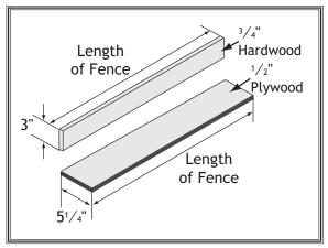
Figure 75. Auxiliary fence dimension.
